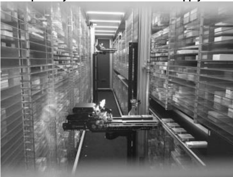
Figure 1. The automated dispensing robot. When medicine labels are requested, or ward stock orders scanned by barcode, one of the robot 'arms' moves along to the required row & column and selects the correct medicine, and outputs it to a conveyer belt system which delivers it to the appropriate output chute. Most medicines are processed into the robot automatically via a 'hopper' that conveys them into the robot for bar code scanning and storage.
